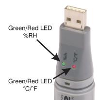
One LED is for temperature measurement, the other is for RH. Each is clearly marked on the logger. To save power, the status indication alternates between the two channels every 10 seconds. So first you will see the status of the temperature logging; 10 seconds later you will see the status of the RH logging and so on.
