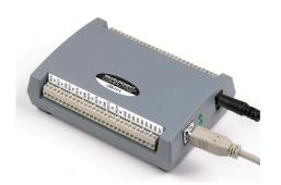
*The USB-3100 Series provides up to 16 voltage/current output channels, with some devices offering high-drive analog outputs.*
