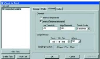
Data logger setup using IQ Wizard is easy. Check the boxes for the samples you'd like to take, select the start method and sample rate, and click OK. Your IQ Logger's ready to go!
