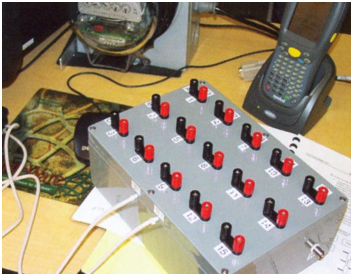
Feeder Study Kit on benchtop with Turtle-equipped end point in background.
