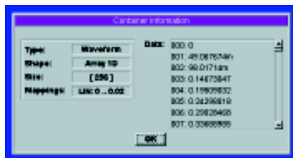
Using HP VEE's line probe makes it easy to examine data as it changes throughout your program.
