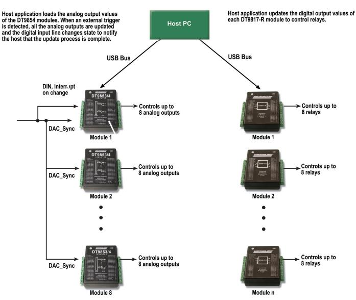
For high-channel count, industrial control applications, use multiple DT9853/54 modules to control analog output signals and multiple DT9817-R modules to control relays.
