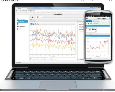
Device-independent operation lets you remotely monitor and control the WebDAQ DT5828 from any device with a web browser.
