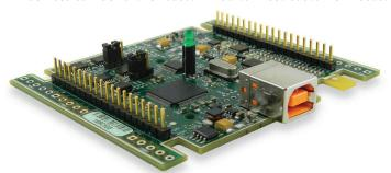
The USB-1208FS-Plus-OEM and USB-1408FS-Plus-OEM have the same specifications as the USB-1208FS-Plus/1408FS-Plus, but in a board-only form factor with header connectors instead of screw terminals.
