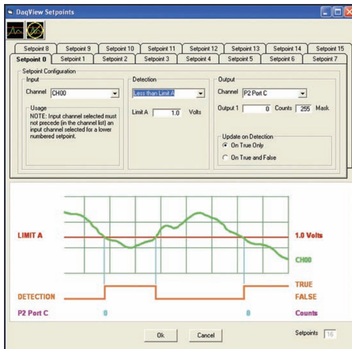
The Setpoint configuration dialog allows the user to configure up to 16 setpoints for their /3000 Series products
