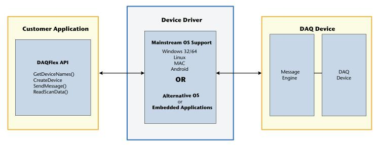
The main components of the DAQFlex software framework are the software API, DAQFlex device driver, and DAQFlex device engine.
