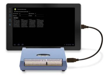
DAQFlex for Android enables development of data acquisition apps that run on Android-based tablets.
