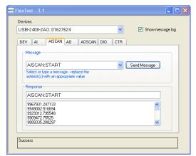
FlexTest is an interactive GUI-based utility that demonstrates how to communicate with a device using the DAQFlex communication protocol and software.
