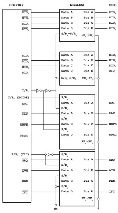
In this example, a high-speed transfer cannot be made, since the bus transceiver is an open collector type.
