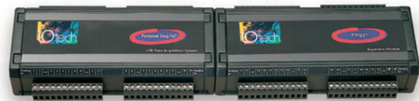
A Personal Daq and a PDQ module simply plug together for additional channel capacity
