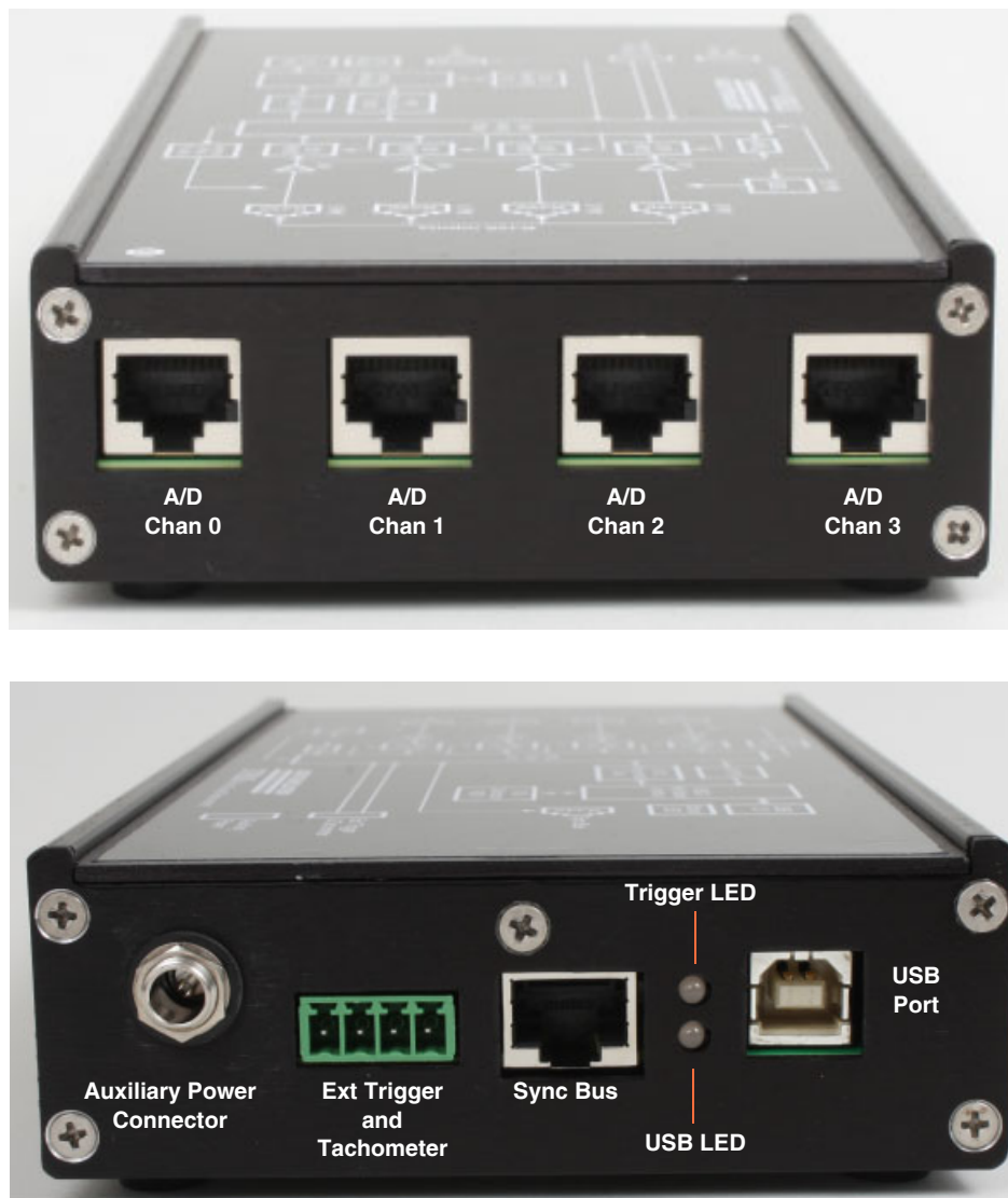
Figure 12: Connectors on the DT9838 Module (Side Views)
