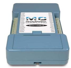
*The BTH-1208LS provides wireless data acquisition up to 1 kS/s and can be hosted by either a Windows-based PC or Android-based device.*
