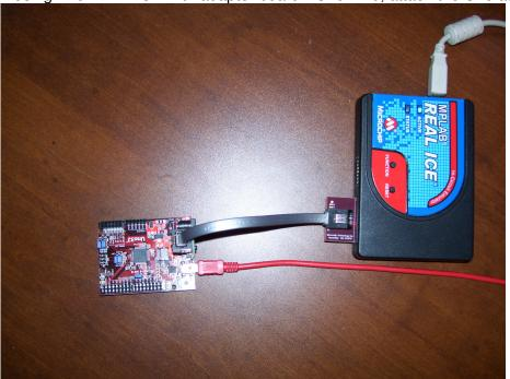
This is how to connect the adaptor board to the Uno32:
