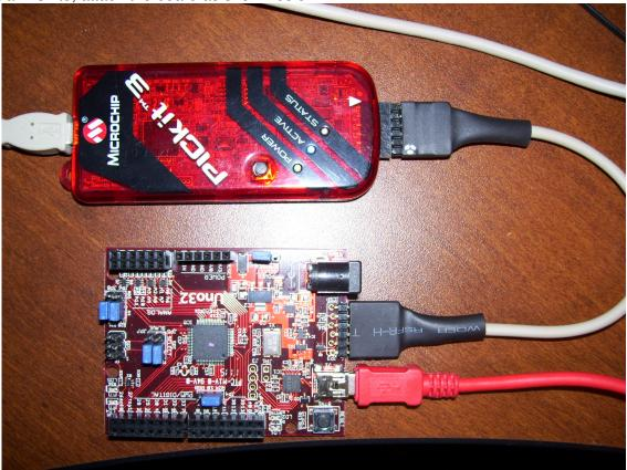
Note: You will need to power the Uno32. It is recommended to use the onboard USB port to power the board.
